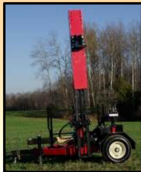
The Hammer and Mast in fully raised position reaches a height of 11' 6" from the hammer to the ground.
