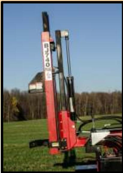
The Mast lifts hydraulically 24 inches. This allows a fast change from 8 to 10 foot posts. This feature also allows a longer hammer stroke for starting 8 foot posts.
