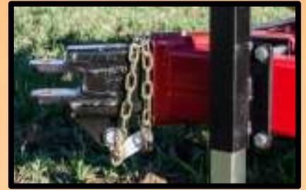
The Mast travels out 16 inches and the tongue travels out 24 inches. This enables the operator to accurately place posts without moving the entire machine.
