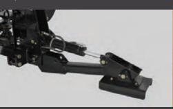
Standard stabilizer pads fit most applications and allow for greater machine stability. A safer operation results by avoiding sudden backhoe movements.
