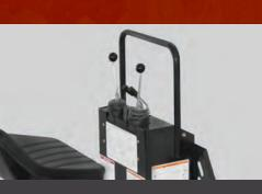
Hydraulic controls with optional joystick for the stabilizer, bucket and boom movements, are all at the operator's fingerprints, eliminating fatigue and making the equipment operation simpler.
