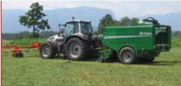
The purpose of the hydraulic driven front rake is to have a baler or loader wagon behind the tractor offering big savings on fuel, working hours and an additional tractor & driver.
