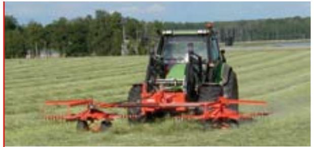
The cam operated rake arms ensure gentle raking into a well formed, fluffy and even swath. The swath width is hydraulically adjustable to make the optimal swath for the pick up on the following machine.
