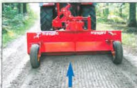
1. Normal forward working position.
