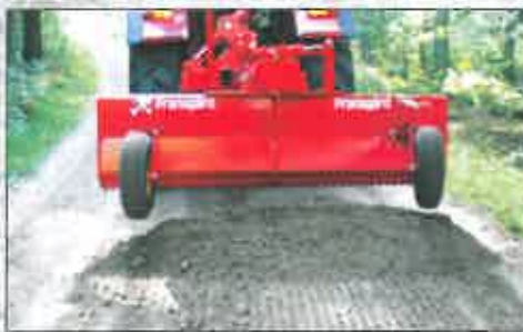
2. The material in front of the blade can be discarded immediately.
