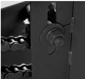
GRYB snowblowers have an easily accessible manual chain idler on the side of the snowblower housing for quick adjustment.
