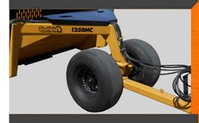
Gooseneck design allows good view of the cutting edge from the cab of the tractor.
