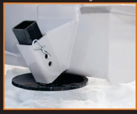
Hydraulic gear driven chute rotator is standard.
