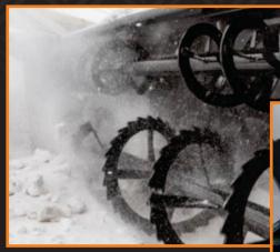
The serrated flighting on the bottom auger is extremely aggressive at eating up that hard packed snow and ice crust.
