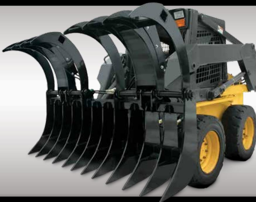
The Root Rake is designed to be invaluable for cleanup operations and is ideal for quickly gathering debris. Afterward the debris can be cleared with an added grapple.
