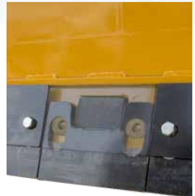
Designed for easy field service, each section of cutting edge uses 2B2N maintenance. This simple 2 Bolt - 2 Nut design makes maintaining each 12" section an easy one person job. Removing the hardware, which holds the retaining plate in place, allows for easy access to the individual components for that section.
