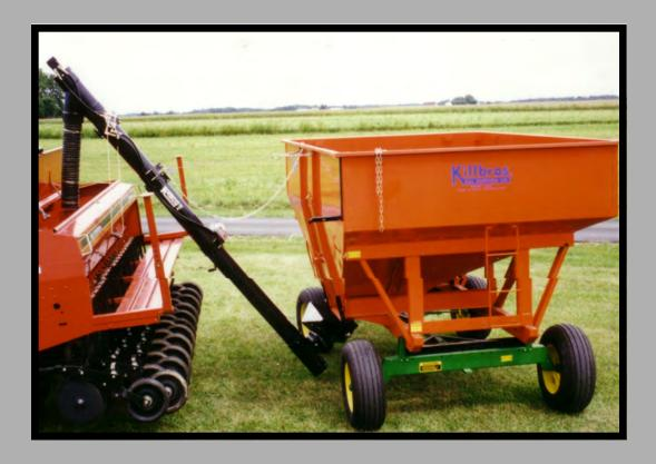
Kasco's Innovative Hopper design allows materials to drop directly into the auger for less seed damage and more positive flow. Different sized hoppers are available, to handle up to a 45" opening on your wagon. A heavy duty winch with built-in brake is included, as is a heavy duty transport bracket to lock the auger in place.
