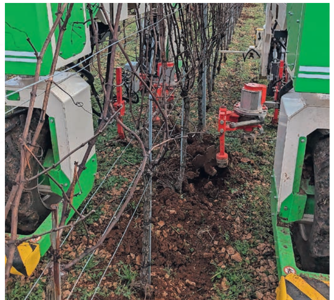
The EVOLT® electric inter-vine developed with Boisselet offers even more accurate adjustment possibilities than your traditional hydraulic inter-vine cultivators.
