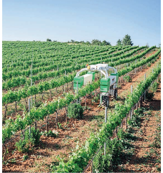
TED adapts to vineyards thanks to two arch heights (6' 7" or 7' 9"). It features the widest arch on the market (3' 5").
