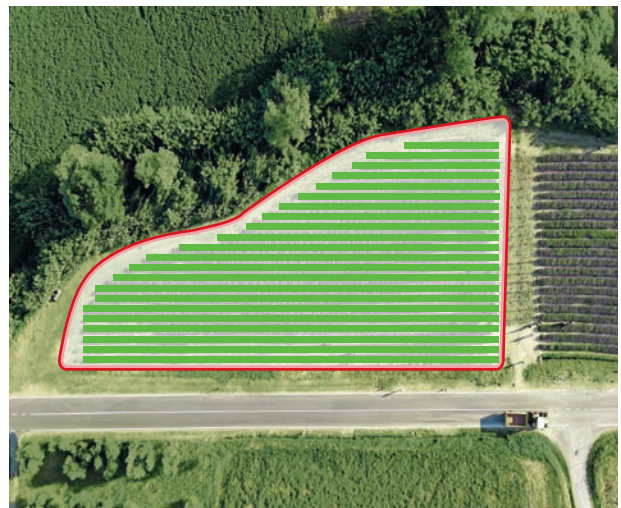
The geofencing prevents the robot from leaving the work area.
