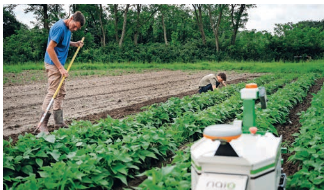
The OZ robot weeds relentlessly to give you more time for tasks that are difficult to mechanize.
