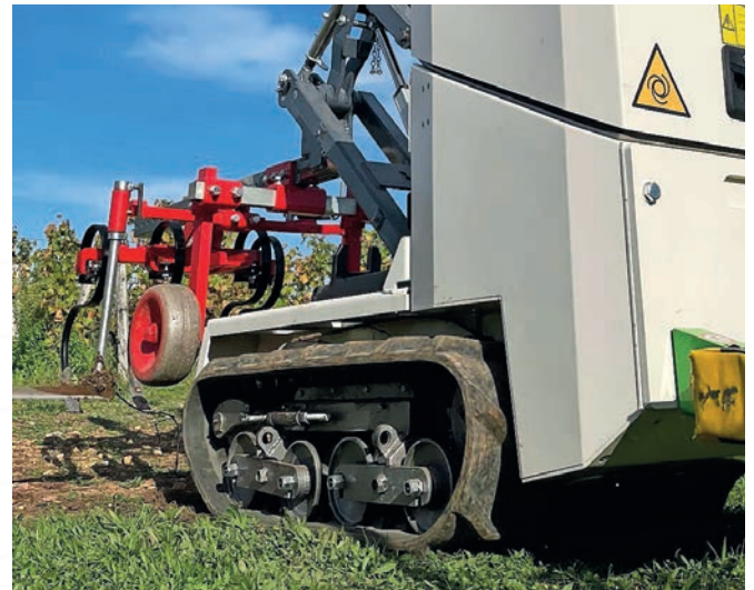
The Boisselet saddle can hold a standard pole or a 3-point lift.
