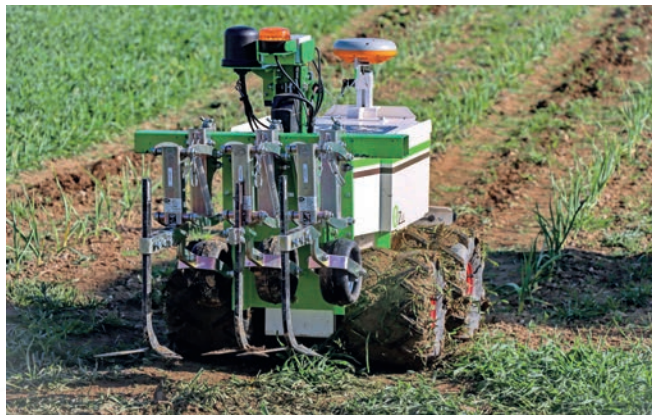
RTK GPS ensures sub-inch accuracy. The work maps produced during sowing or furrow tracing are used for the entire technical itinerary.
