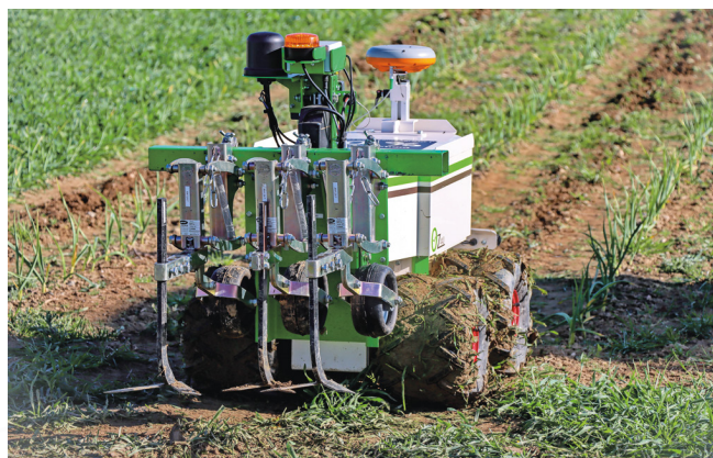
RTK GPS ensures centimeter accuracy. The work maps produced during sowing or furrow tracing are used for the entire technical itinerary.
