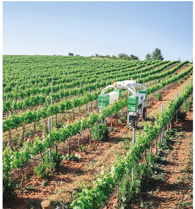
TED adapts to vineyards thanks to two arch heights (2.00 m or 2.35 m). It features the widest arch on the market (1.05 m).
