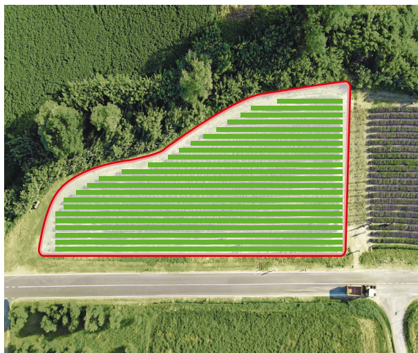
The geofencing prevents the robot from leaving the work area.
