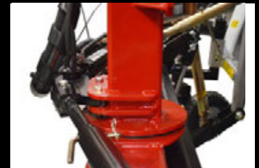
DOUBLE SHEAR ANGLE CYLINDER MOUNT
