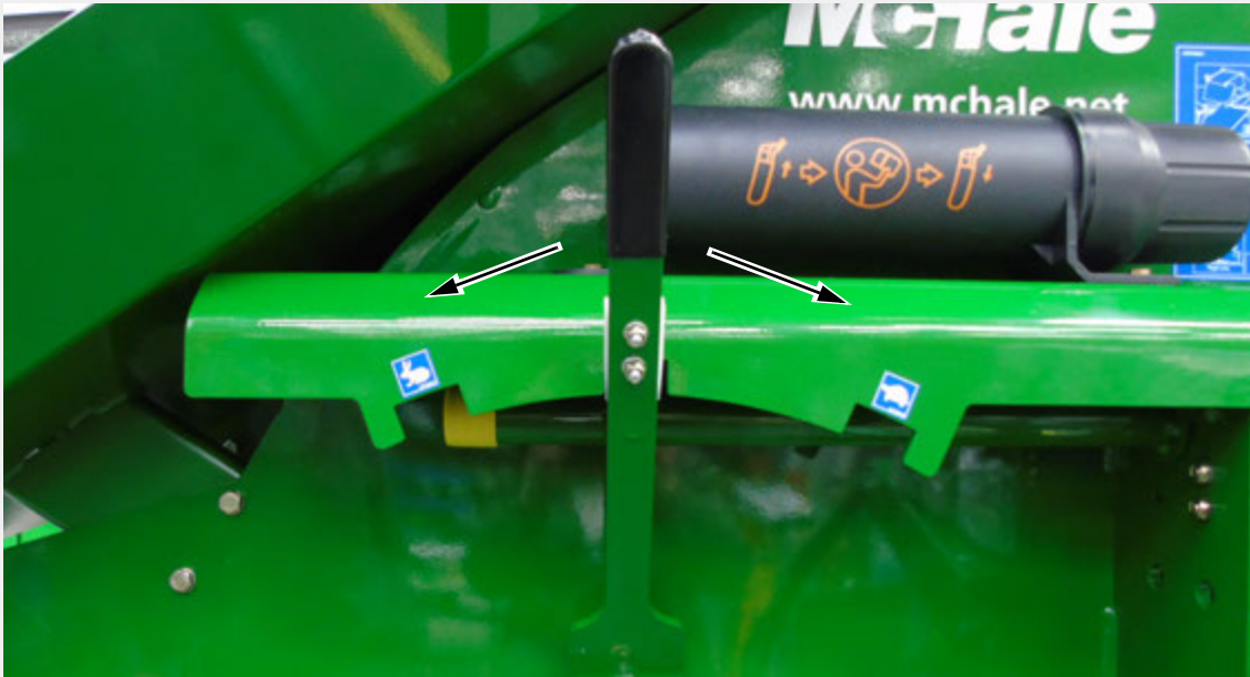
Gear selection (shown in neutral)
