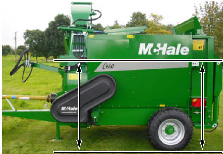
Machine to be horizontal to the ground
