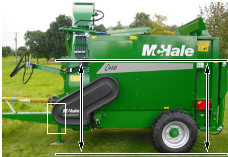
Machine to be horizontal to the ground
