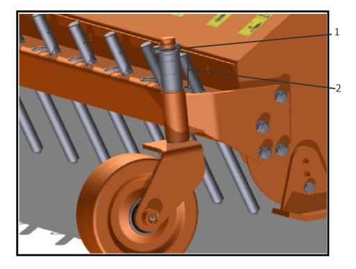
Depending on the different position of the spacers on the shaft, it is possible to set fivedifferent cutting heights: 70-76-89-114 and 145 mm.
