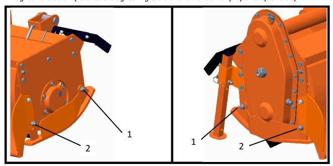
When finished, verify that both skids are at same level, and check if the front of the tiller is leveled to the back, when lowered to the ground. Adjust with the 3-point top link if necessary.
