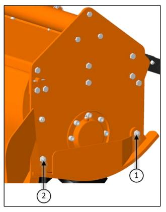
When finished, verify that both skids are at same level, and check if the front of the tiller is leveled to the back, when lowered to the ground. Adjust with the 3-point top link if necessary.
