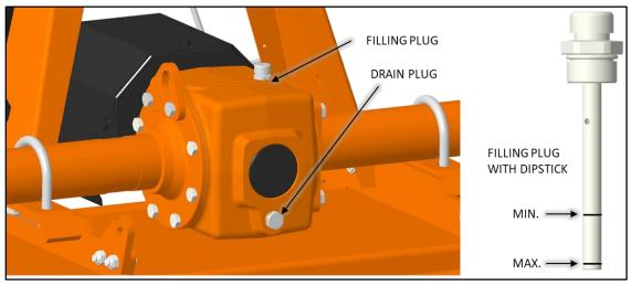
If the sign is below the minimum, fill up oil till restore the correct level.
