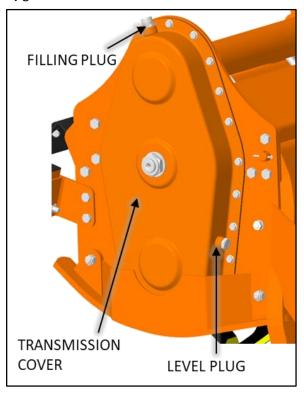
Check the oil level every 50 hours, making sure it reaches the level plug on the transmission cover. If the oil is below this level, fill up oil till restore the level.
