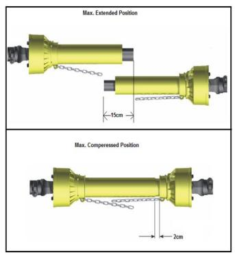
A driveshaft too long may cause structural damages to the tractor and machine. If the driveshaft is too long, it may be adapted by removing it and shortening the tubes according to the instructions provided by the Manufacturer in its use and maintenance manual.
