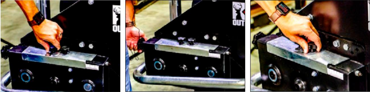
**#5** After verifying that your settings are correct, seed is in all of the seed cups, and the seed catching device is in place, use a piece of tape or marking as a set position on the cultipack roller.
