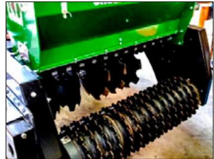
**#1** You will need to find a box or tray that will fit across the width of the seeding elements to catch all of the seed falling from the machine during the calibration process. You will want to mount the box or tray as close to the bottom of the seeding element openings as possible to help you not lose any seed.
