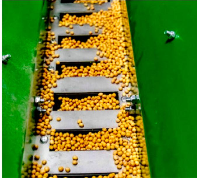
**#3** Using the SEED SETTING CHART to get your base setting for the seed you will be planting. On the right side of the Ground-Breaker, you will adjust the Gate Opening number from 0 - 3 by loosening the knob, moving the bar to the correct number, and tightening back the knob.
